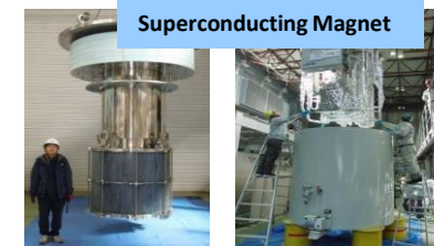
13 T, \phi 700 mm Solenoid Coil
